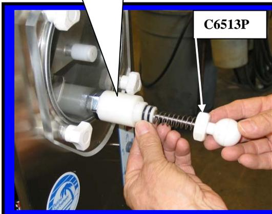
Installing **Faceplate** onto front of Machine.
