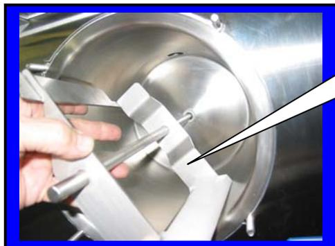
Step 7: Install beater bar assembly C6527 into cylinder.
