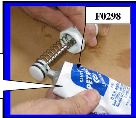
Installing **Plunger Assembly** into Faucet body
