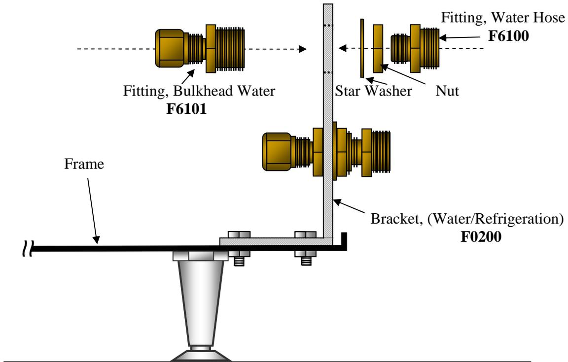
1. Insert the water bulkhead fitting P.N. F6101 through the bracket hole.
