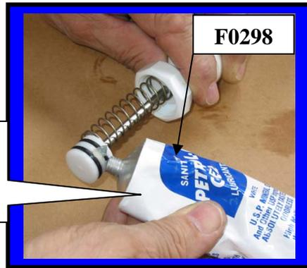
Installing **Plunger Assembly** into Faucet body
