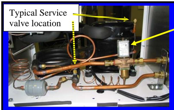
Valves automatically open on pressure increase, close on pressure decrease. **Adjustment:** To raise valve opening point, turn adjusting screw, on top of valve, counter-clockwise. To lower operating point, turn clockwise. Opening point of valve should be raised just enough to cause valve to close during compressor stand-by periods.
