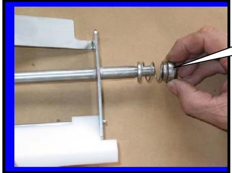
Step 5: Install spring seal F0355
