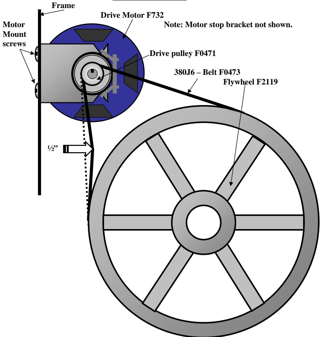
1. To increase belt tension, loosen the 4 motor mount screws and pry the entire motor assembly *up* until the belt is snug. Re-tighten the motor mount screws.
