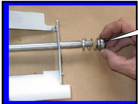
Step 5: Install spring seal F0355
