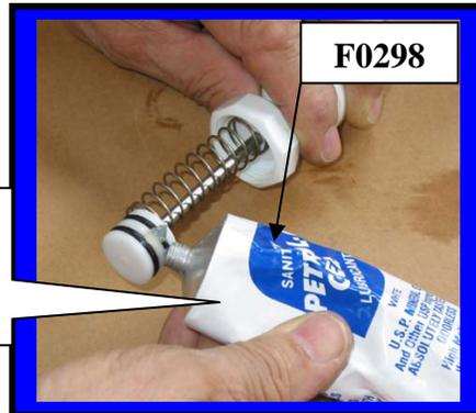
Installing **Plunger Assembly** into Faucet body
