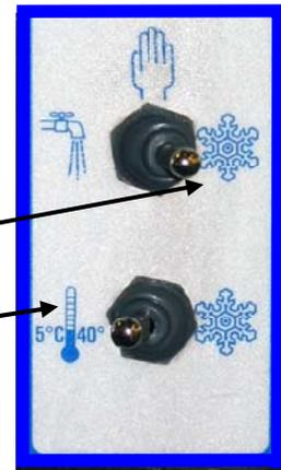
**Cooling Operation** – Top switch on **snowflake**, Bottom switch on **thermometer** symbol. Machine will automatically come on whenever necessary to keep mix cooled to 5°C/40°F - used primarily for overnight storage of mix remaining in the machine.
