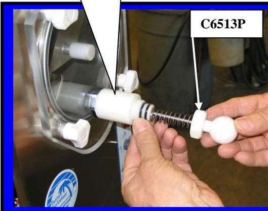
Installing large **Faceplate** onto front of Machine.
