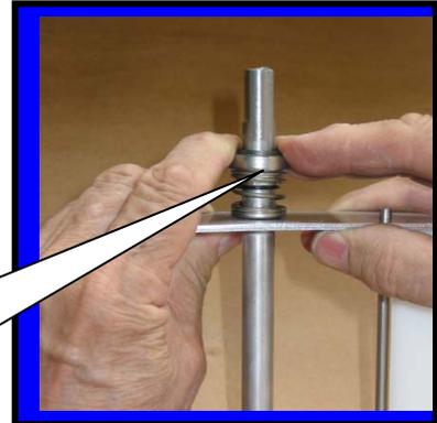
Step 6: Squeeze and release spring. Be sure the spring returns to normal before installing into machine.
