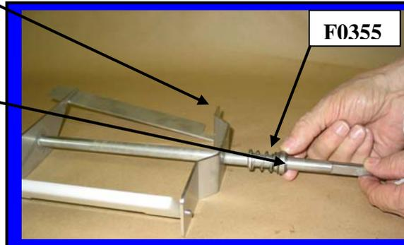
The **black carbon ring** must be facing the end of the beater bar so it will be in direct contact with the white ceramic seal inside the cylinder when the beater bar is re-installed.
