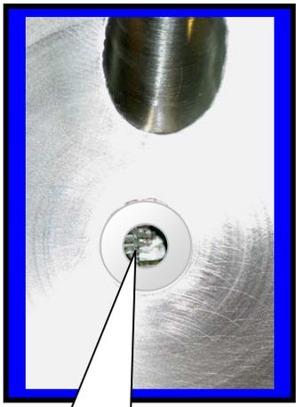
Push brush all the way in until it can be seen in the middle of the ceramic ring
