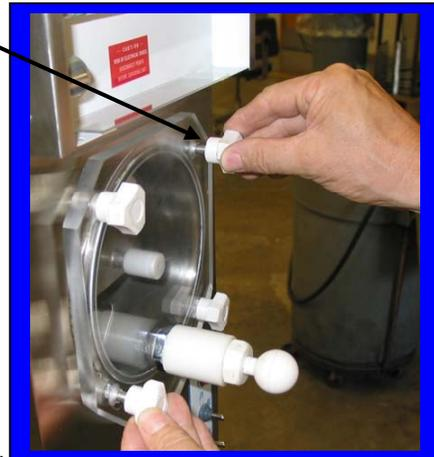
**NOTICE:** Do not unscrew faucet body from faceplate to clean. (Leak free service after disturbing the Teflon seal cannot be assured).
