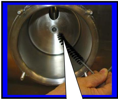
Insert short brush **F0326** into the center of the ceramic ring to remove any grease or dried product.
