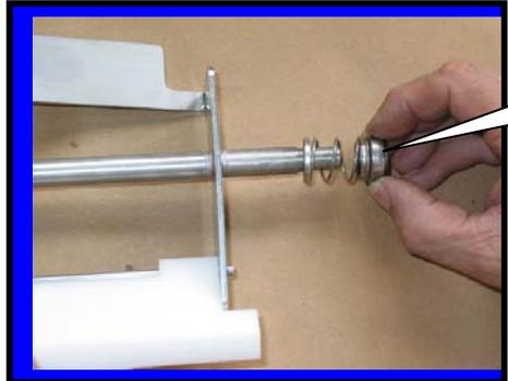
Step 5: Install spring seal F0355
