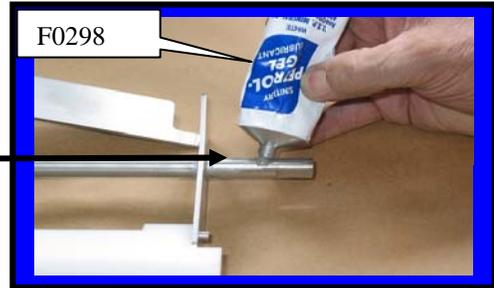
**NOTICE:** The **black carbon ring** must be facing the end of the beater bar so it will be in direct contact with the white ceramic seal inside the cylinder when the beater bar is re-installed. **This is a dry seal and must be kept free of lubricants.**
